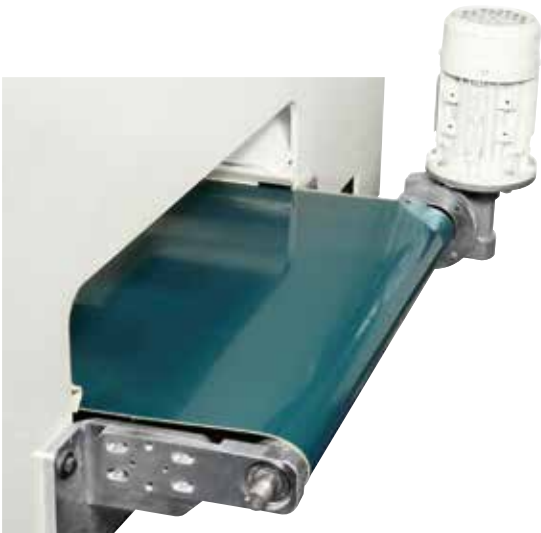
Collecting belt for carrying away machining waste and shavings.
