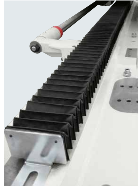
Bellows for protection against abrasive dust applied on moving parts. They prolong life of mechanical parts and significantly reduce maintenance.
