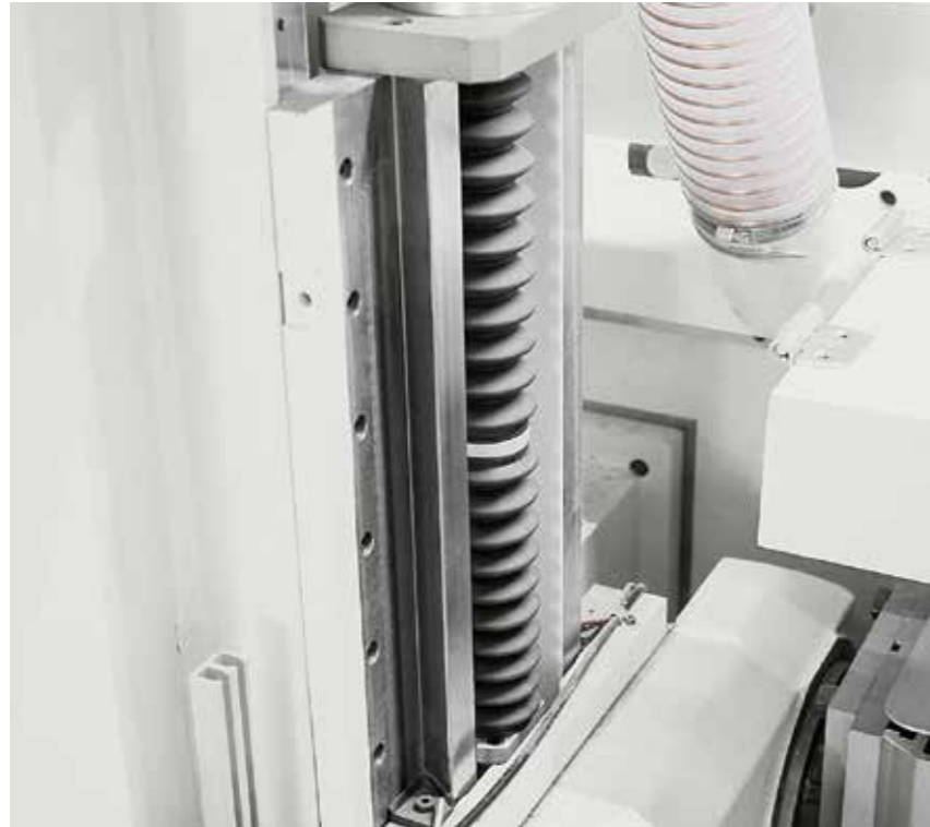
Bellows for protection against abrasive dust applied on moving parts. They prolong life of mechanical parts and significantly reduce maintenance.
