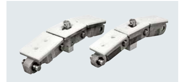
Rolling feed chains 43, 60 or 75 mm wide to process workpieces with minimum width 90, 140 or 170 mm*
