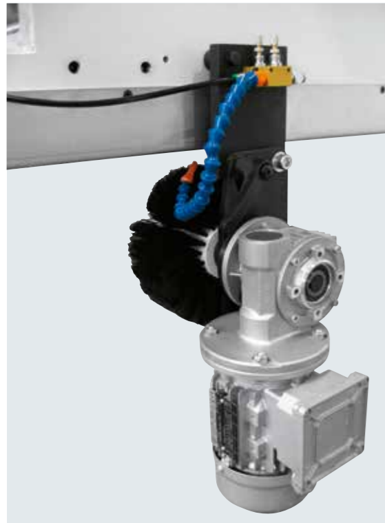
Pressurization and rotating brushes for the cleaning of chain tracks.
