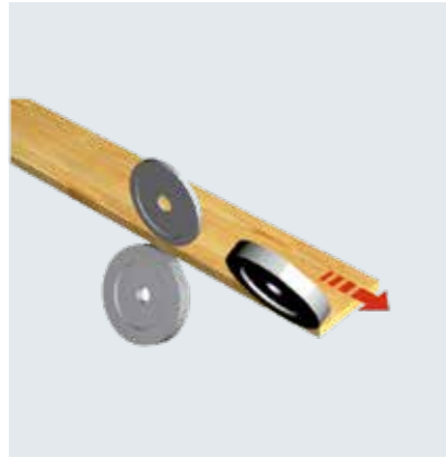
Edge trimming and chamfering unit for top, bottom or both edges.
